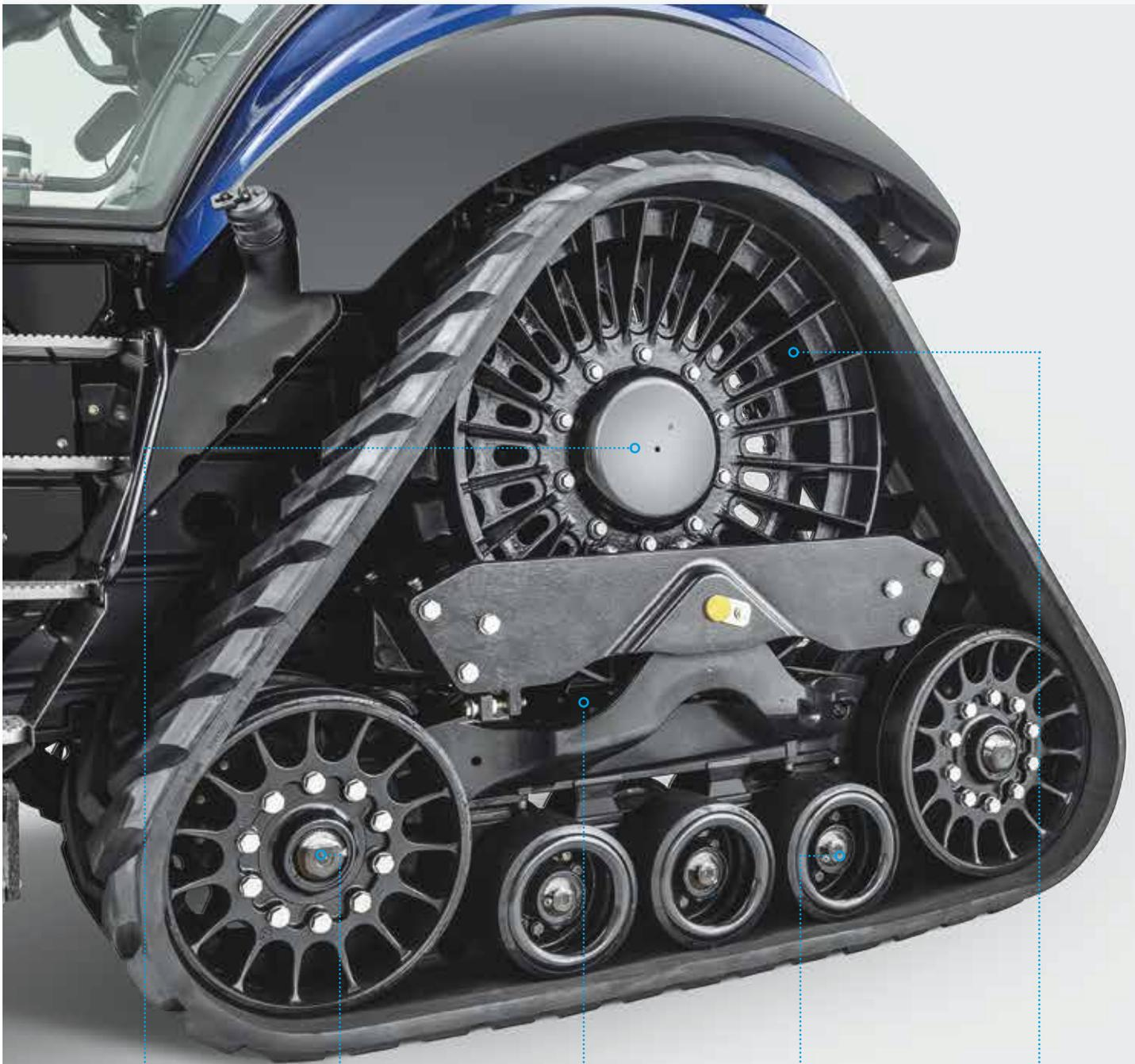
Ductile cast iron drive wheel
